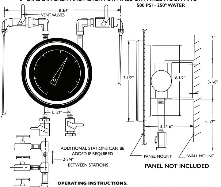
IN ORDER TO READ METER, AIR MUST BE PURGED FROM VENTURI THROUGH METER
